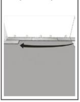
6. IMPORTANT! Use rubber mallet and tapping block to tap long edge of plank to ensure a tight fit. ANY GAPPING CAN COMPROMISE THE LOCKING
