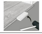
2. Use rubber mallet and pull par to lock short end of plank.
